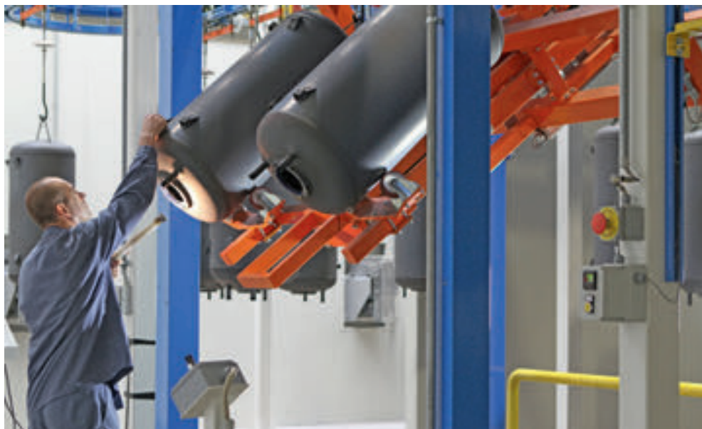
Boiler inners undergo a visual check before the outer casing is added.
