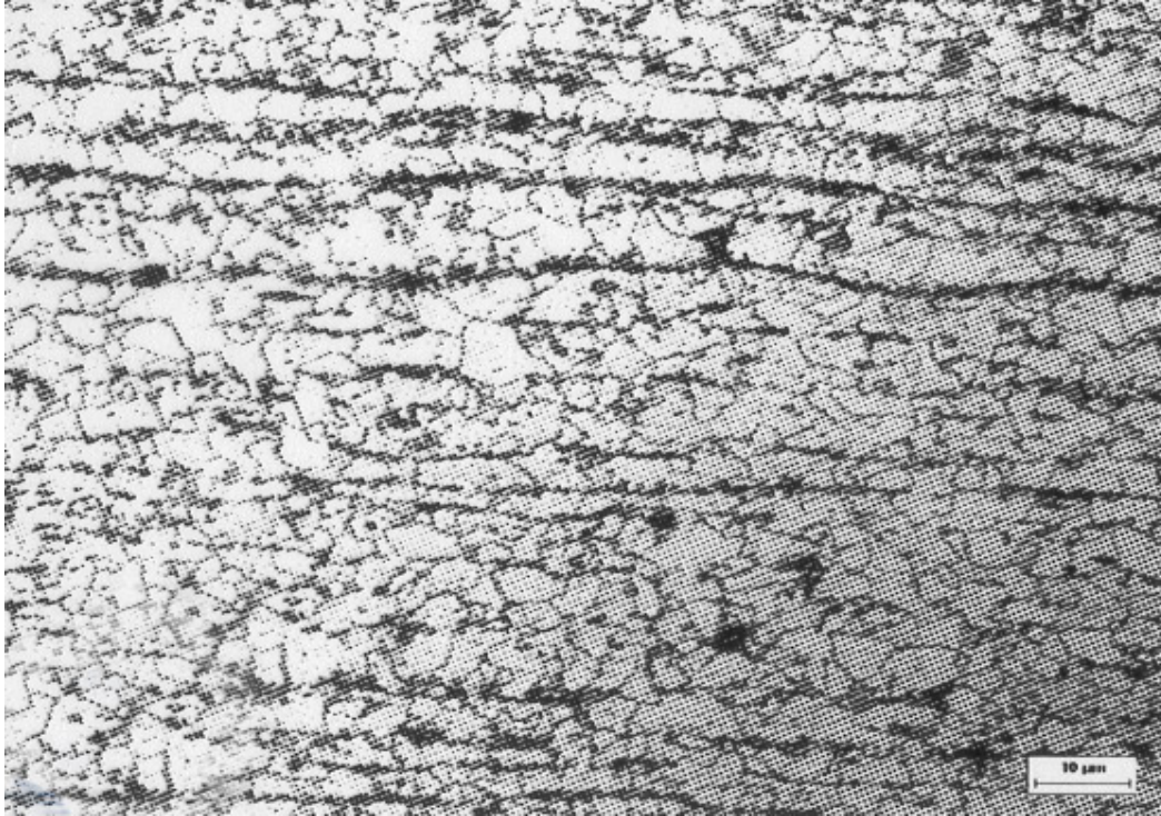
HDGA-HFT 590 containing ferrite, pearlite and bainite.
