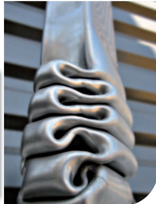
Usibor® 1500P steel, a high strength steel grade that plays a key role in the weight reduction of many new bodies-in-white, has long been produced exclusively in Europe. But since it was 'cloned' in 2009, it has also been available on the North American market.
