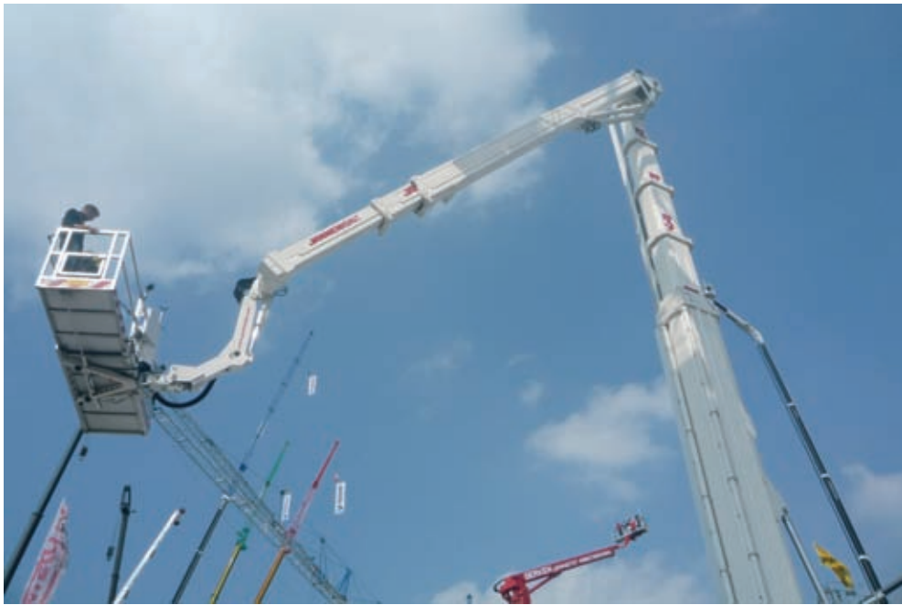
The newly developed S700MC grade is not only suitable for trailers. Typical applications for S700MC include telescopic cranes, tippers and truck chassis.
