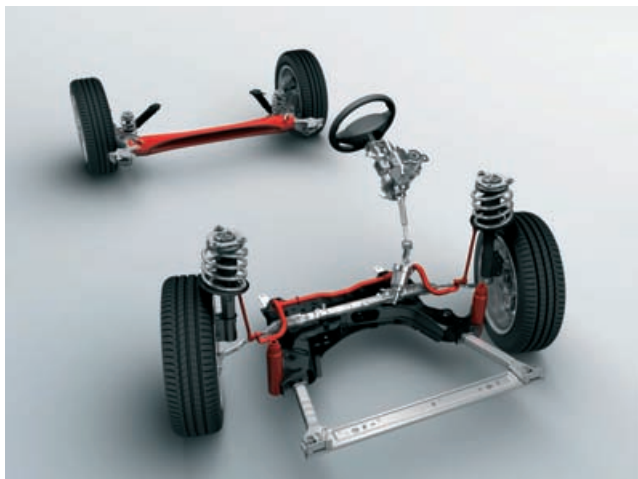
Sub assembly for the Renault Mégane III showing tubular twist beam (in red on rear axle), shock dampers (red, front group), front cradle (black, front group), and crash component (silver, front group)
