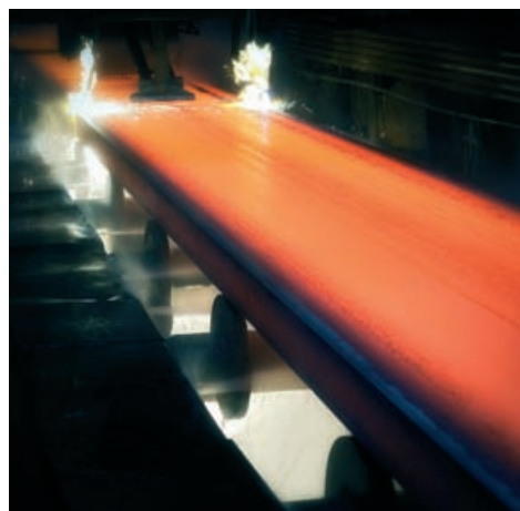
Slab oxycutting at Fos-sur-Mer. Refined ladle metallurgy techniques and finely tuned continuous casting conditions enable us to reach a very low level of segregation, qualifying our products for sour service. (image: Alain Sauvan)
