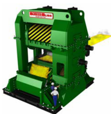
In late 2010 our Bremen mill unveiled the world's largest crop shear which can shear transfer bars up to 76 mm thick prior to finish rolling. The crop shear also opens up the possibility of creating new properties. (image courtesy Butech Bliss, USA)
