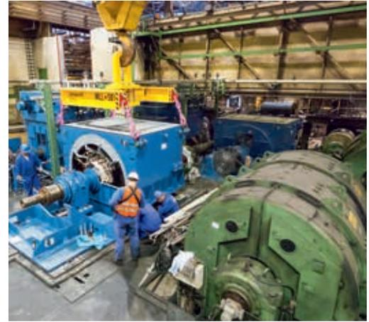
Assembly of the new synchronous motor for the cold strip tandem mill (left) and an old direct current motor (right).
